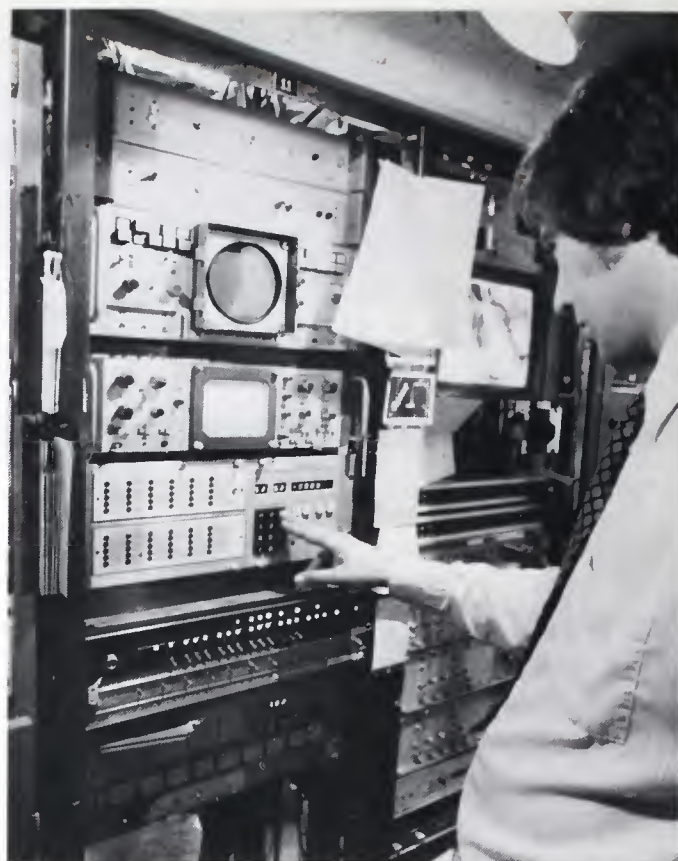
Figure 7. Charles Rose, KPIX studio technical supervisor, examines the remote control unit in downtown studio master control room. Unit enables any of 26 communications functions to be dialed up remotely, allowing picture quality, waveforms and other functions to be inspected.
