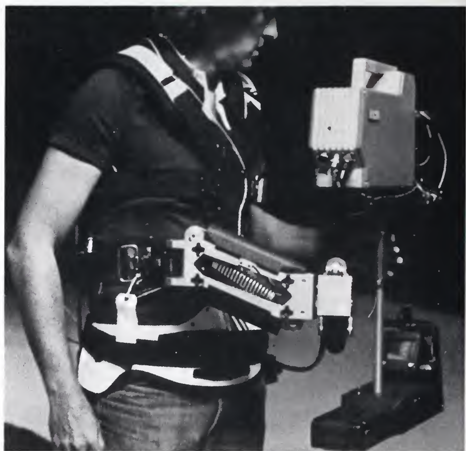
The Steadicam by Cinema Products was demonstrated with wild exuberance around their booth at the SMPTE convention in New York. Shown here with an RCA TK-76 ENG camera, the Steadicam is a unique and revolutionary camera stabilizing system designed to damp out camera vibrations and motion effects for a steady picture.
